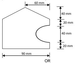
7 Calculate the moment of inertia of the section shown in figure below about xx and yy axis through the centroid.
